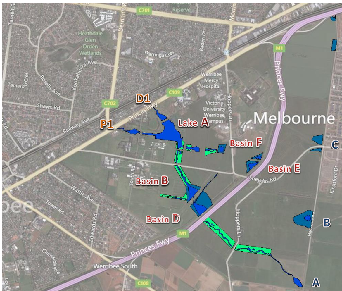
Figure 3.5: Overview of redesigned stormwater treatment train within the East Werribee Precinct
