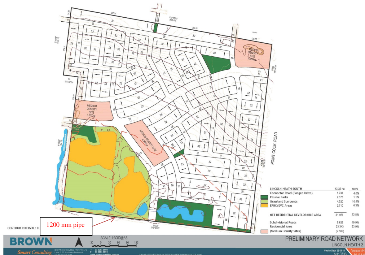
Figure 3 Preliminary road network and main drainage layout.
