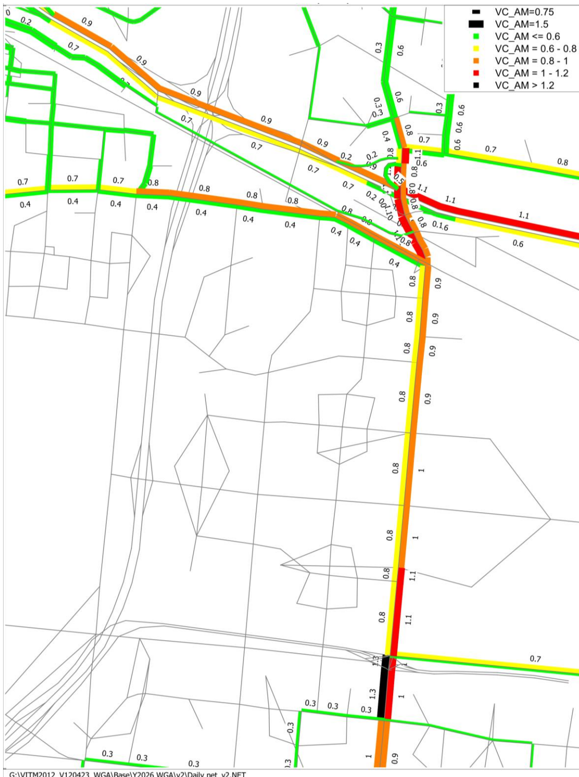
Figure 14: 2026 AM volume to capacity ratios
