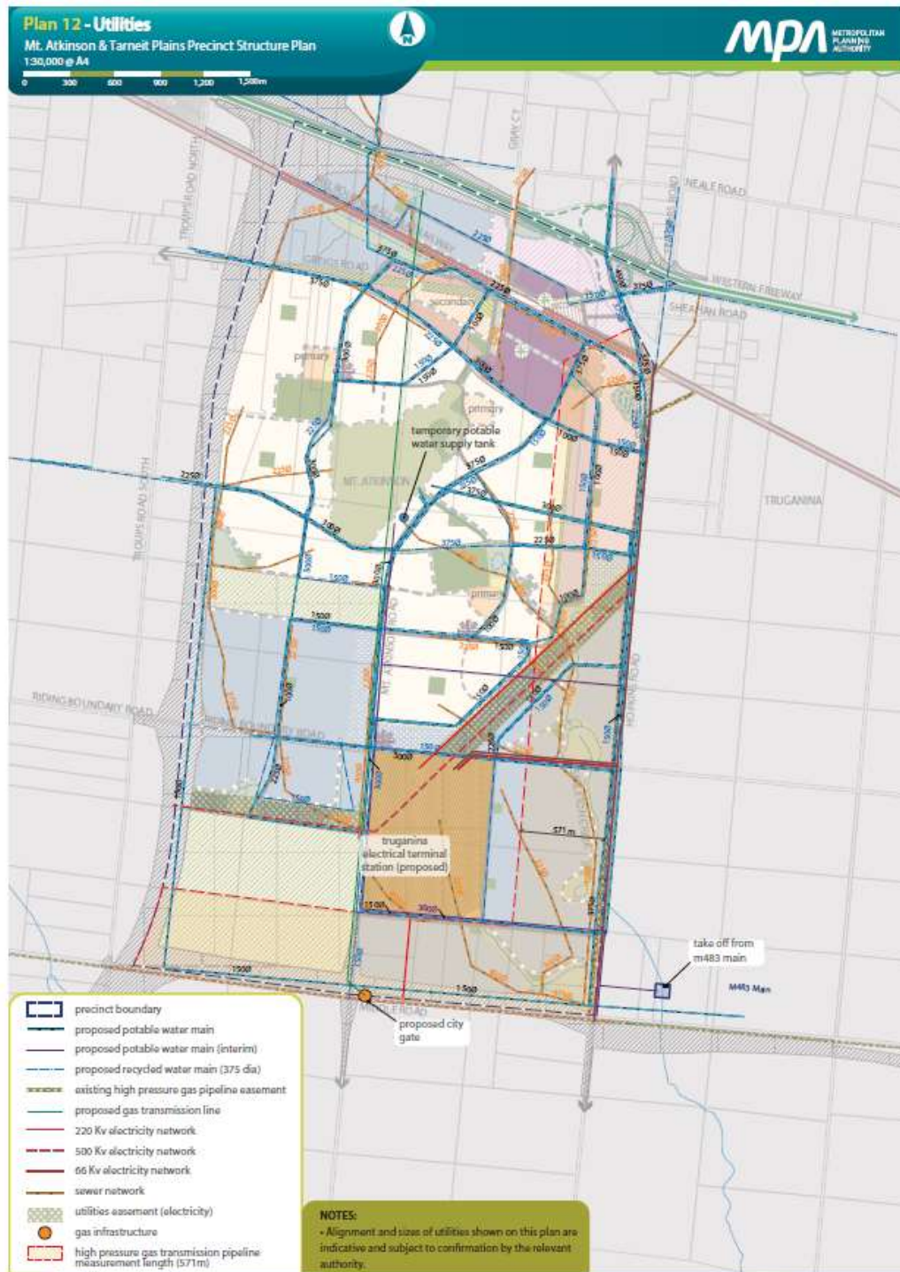
Figure 17 – Plan 12 of the exhibited draft PSP, showing the gas pipeline 'measurement length'.
