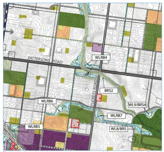
Figure 3 - Location of stormwater management infrastructure in the Clyde Creek PSP near the corner of Tuckers Road and Pattersons Road (Mel Ref: 135 D8).
