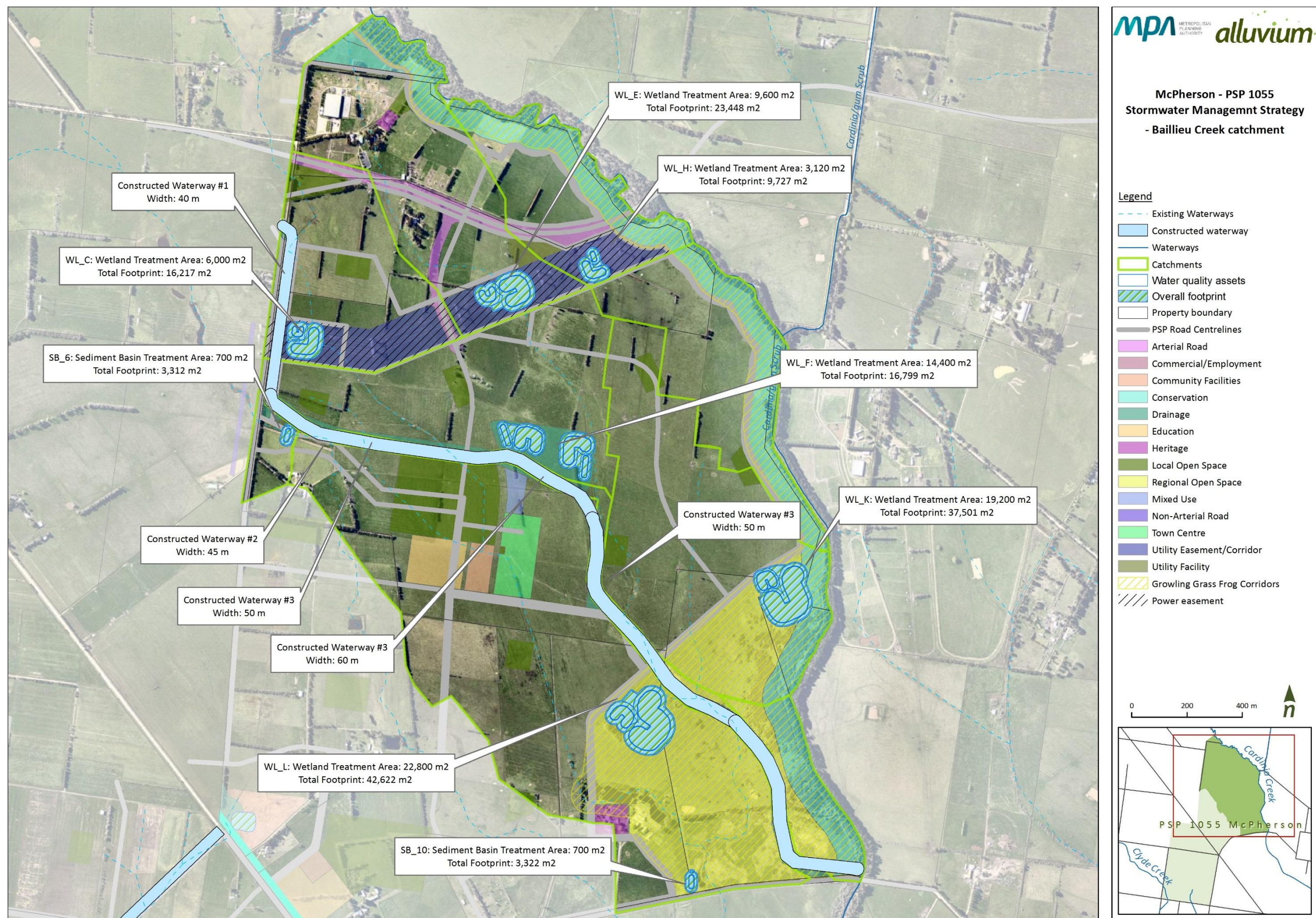
Figure 17. Recommended layout of McPherson PSP (northern section) surface water management strategy
