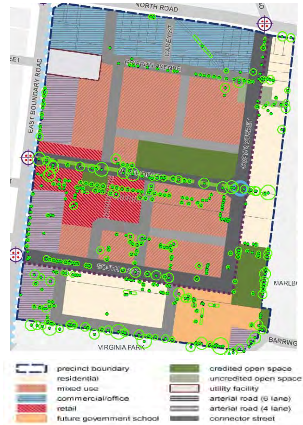
Figure 19: Concept design with tree and TPZ locations overlaid
