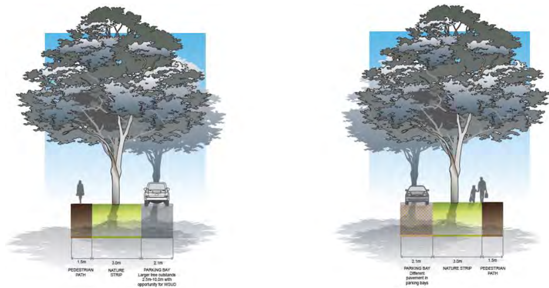
Figure 4.7: Indicative Cross-Section - Local Access Level 1 (16m)
