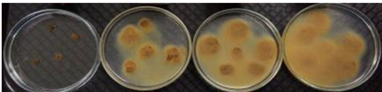
Figure 2.1: Examples of soil aggregates subject to the Emerson Aggregate Test, showing nil dispersion on the left with increasing levels of dispersion to the right (Armstrong 2019).
