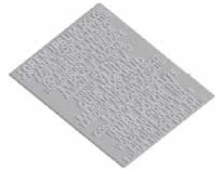
Laser etched text into paving stone
