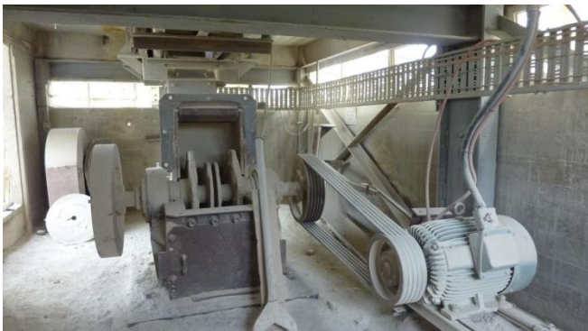
Figure 68 Top level of the Road Metal Plant: the Jaques jaw crusher in not original
