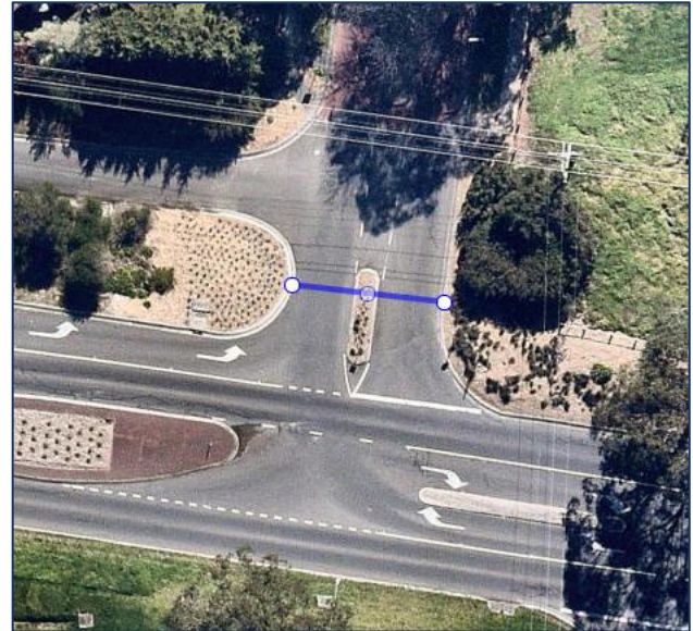
Figure 5-2 Left: Tube Counter Placement on Lakeview Drive (West) – Aerial View Right: Tube Counter Between Hull Road Carriageway and Shared Use Path – Aerial View
