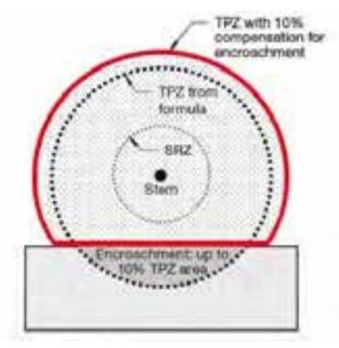
Figure 7: Example of minor TPZ encroachment and compensatory offset (image from AS 4970-2009).
