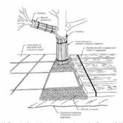
Figure 10: Example of trunk, branch and ground protection (Source: AS 4970-2009).
