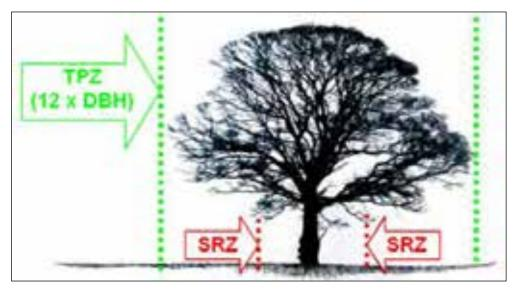
Figure 6: The SRZ = minimum volume of roots required for tree stability. Image from Biddle 1998.
