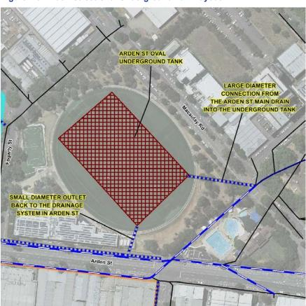
Figure 4.6: Arden Street Oval Underground Tank layout
