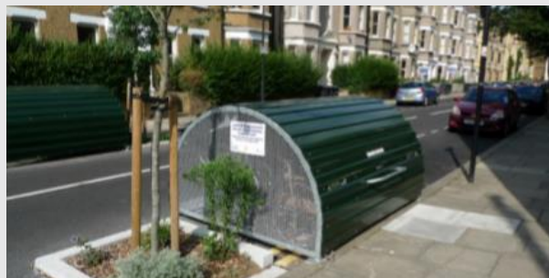
Haringey London, UK Bike Hanger - bike lockers for six bicycles that occupies less than one parking space. These are oversubscribed
