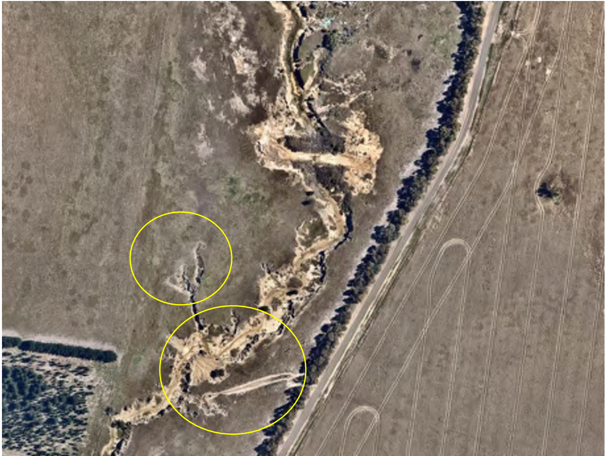
Figure 5-2: Tunnel erosion adjacent to Kalkallo Creek
