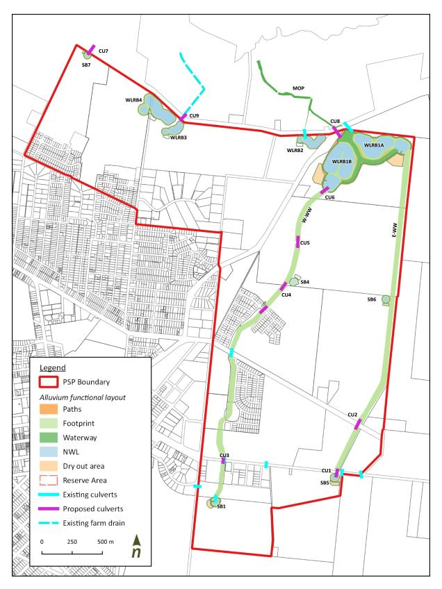
Figure 26. Overall layout of stormwater assets for the PSP – Alluvium 2021
