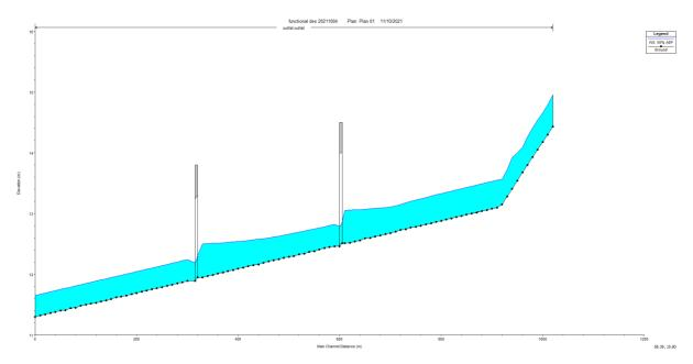
Figure 50. 50% AEP water surface elevation along the waterway alignment with culverts unimpeded
