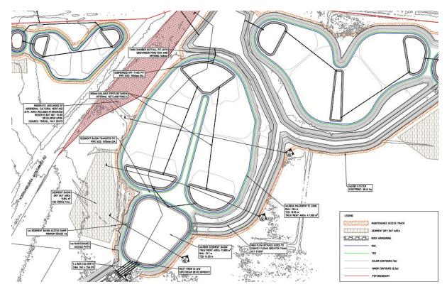
Figure 60. Plan view of the designed wetland structure WLRB1B (DCP ref WL-01/RB-01) (west)
