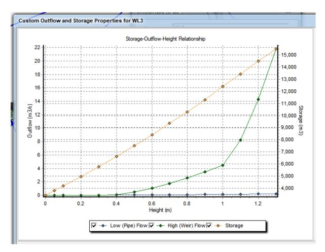
**Figure 65.** Stage-storage-discharge relationship for WLRB3 (DCP ref WL-03)
