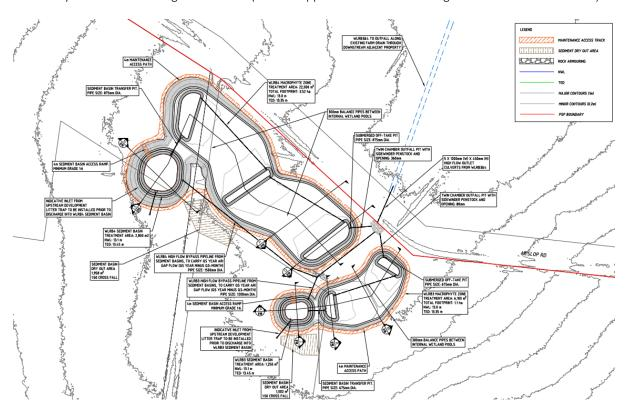
Figure 64. Plan view of the designed wetland structure WLRB3 (DCP ref WL-03)
