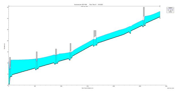
**Figure 34.** 1% AEP water surface elevation along the waterway alignment with culverts unimpeded
