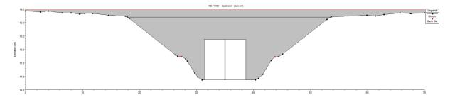
Figure 32. Upstream Centennial Dr cross section (looking downstream)
