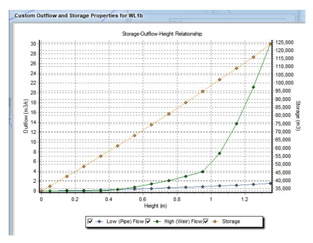
Figure 61. Stage-storage-discharge relationship
