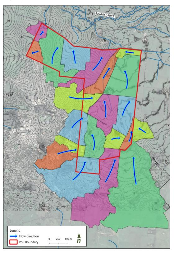
**Figure 16.** Stormwater drainage sub-catchments across the PSP area (Engeny delineations, 2021)
