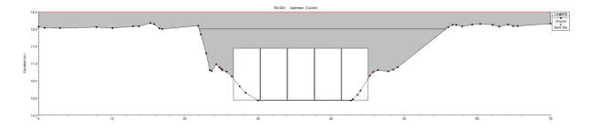
**Figure 33.** Upstream culverts 4, 5, 6 cross-sections (looking downstream)
