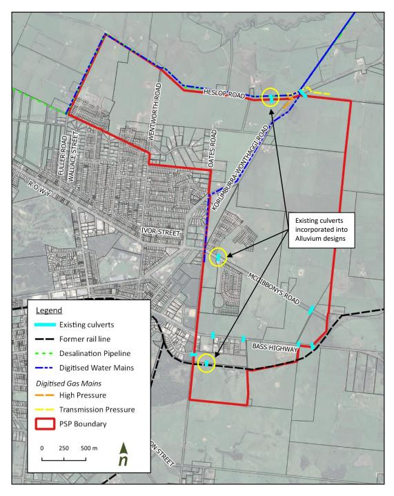
**Figure 13.** Existing services and infrastructure in PSP area. Water mains digitised based on images by South Gippsland Water, gas mains digitised based on images by Multinet Gas - based on data provided 27/08/2021)
