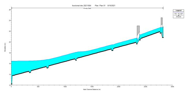
$\textbf{Figure 41.}\ 1\%\ AEP\ water\ surface\ elevation\ along\ the\ waterway\ alignment\ with\ culverts\ unimpeded$
