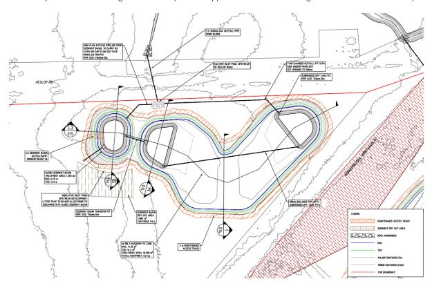
Figure 62. Plan view of the designed wetland structure WLRB2 (DCP ref WL-02)
