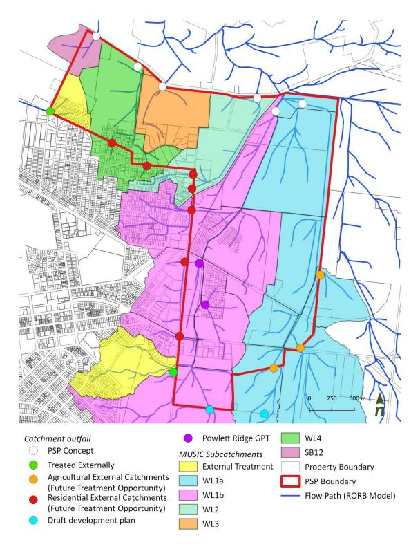
Figure 15. Map of drainage catchments and respective outfalls indicating ideal treatment asset locations within/beyond PSP.
