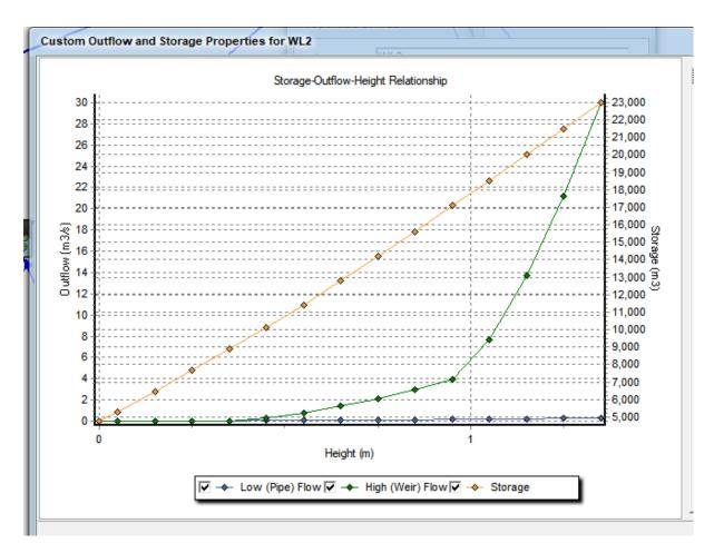
Figure 63. Stage-storage-discharge relationship
