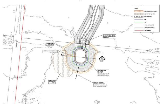
**Figure 68.** Plan view of the designed wetland structure SB1(DCP ref SB3)
