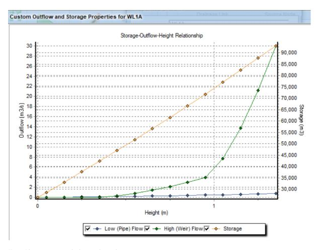
Figure 58. Stage-storage-discharge relationship
