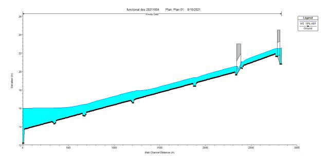
Figure 43. 10% AEP water surface elevation along the waterway alignment with culverts unimpeded
