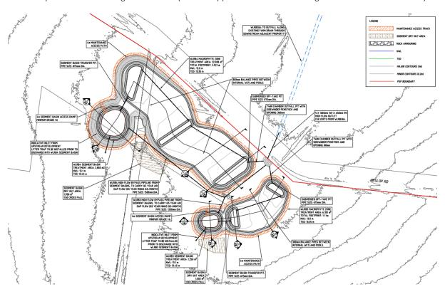
Figure 66. Plan view of the designed wetland structure WLRB4 (DCP ref WL-04)
