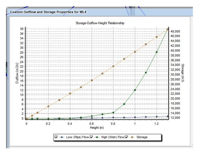
Figure 67. Stage-storage-discharge relationship
