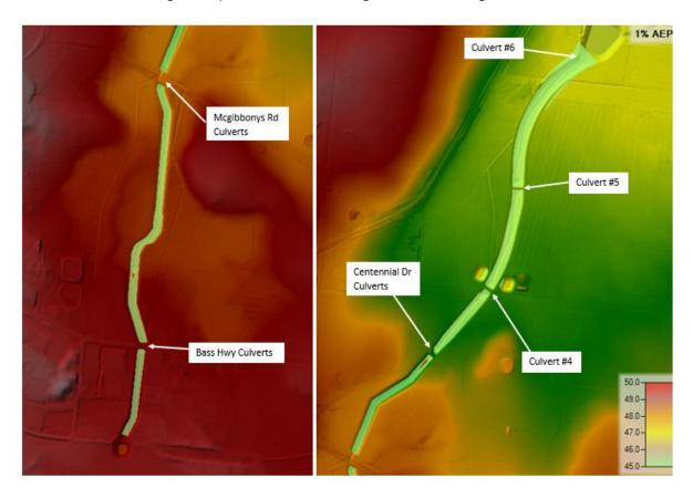
**Figure 38.** Average shear stress map through constructed waterway (in N/m²)
