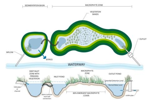
Figure 23. Typical concept layout of a treatment wetland (source: Constructed Wetlands Design Manual, Melbourne Water)
