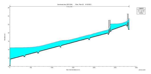
**Figure 42.** 1% AEP water surface elevation along the waterway alignment with culverts 50% blocked
