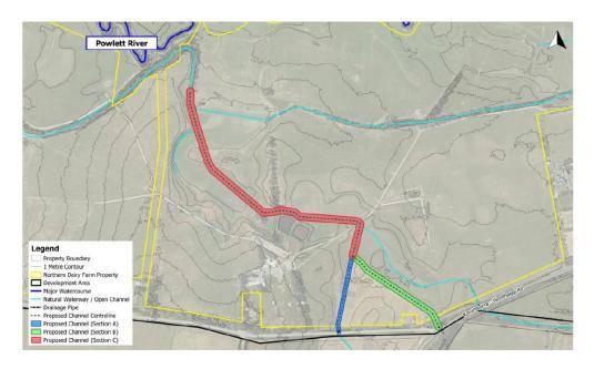
Figure 25. Planned mitigation works to reduce flooding on the subject property – 465 Heslop Road (source: Engeny, 2021)
