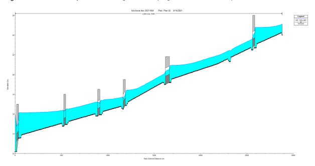
**Figure 37.** 10% AEP water surface elevation along the waterway alignment with culverts 50% blocked
