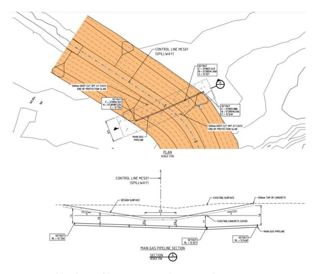
**Figure 47.** Proposed channel crossing of the gas transmission main (Engeny, Aug 2021)
