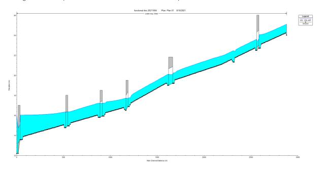
Figure 36. 10% AEP water surface elevation along the waterway alignment with culverts unimpeded
