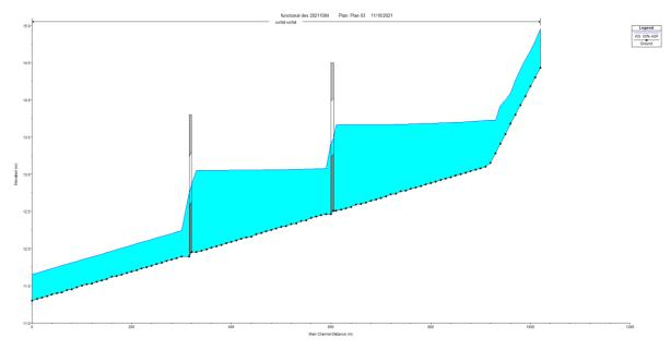
Figure 51. 50% AEP water surface elevation along the waterway alignment with culverts blocked
