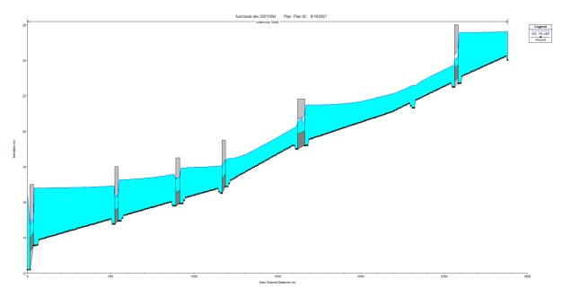
Figure 35. 1% AEP water surface elevation along the waterway alignment with culverts 50% blocked
