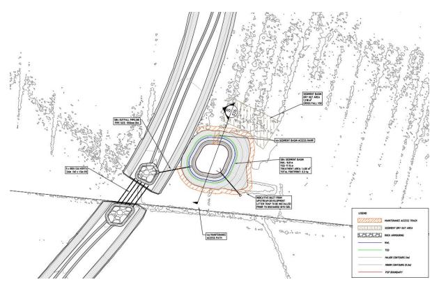
**Figure 69.** Plan view of the designed wetland structure SB4 (DCP ref SB7)
