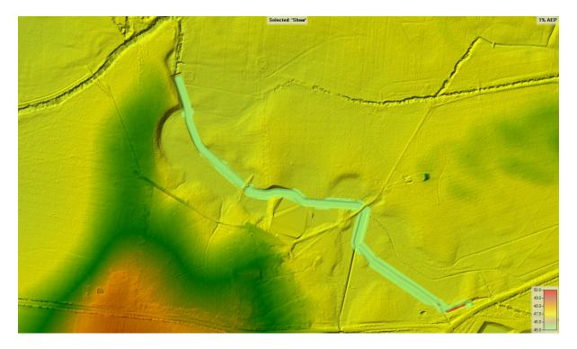
**Figure 52.** Average shear stress map through constructed waterway (in  $N/m^2$ ) – note red grading near WLRB1 (DCP ref WL-01/RB-01) outfall to MOP.
