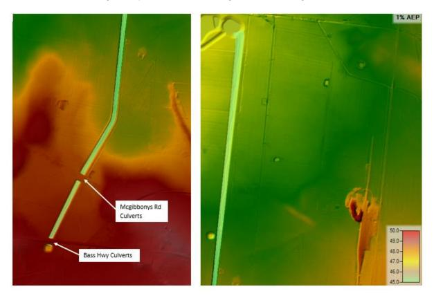
**Figure 45.** Average shear stress map through constructed waterway (in N/m²)
