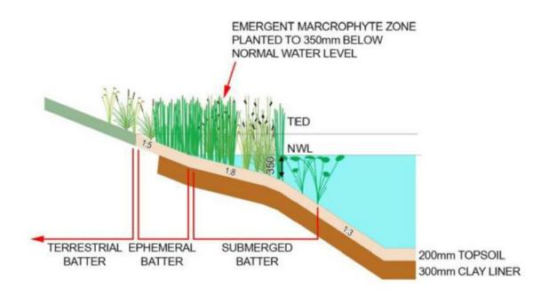
**Figure 56.** Edge treatment for batter slopes (Melbourne Water 2014)
