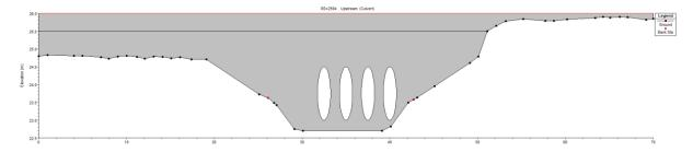
Figure 30. Upstream Bass Hwy design cross section (looking downstream)
