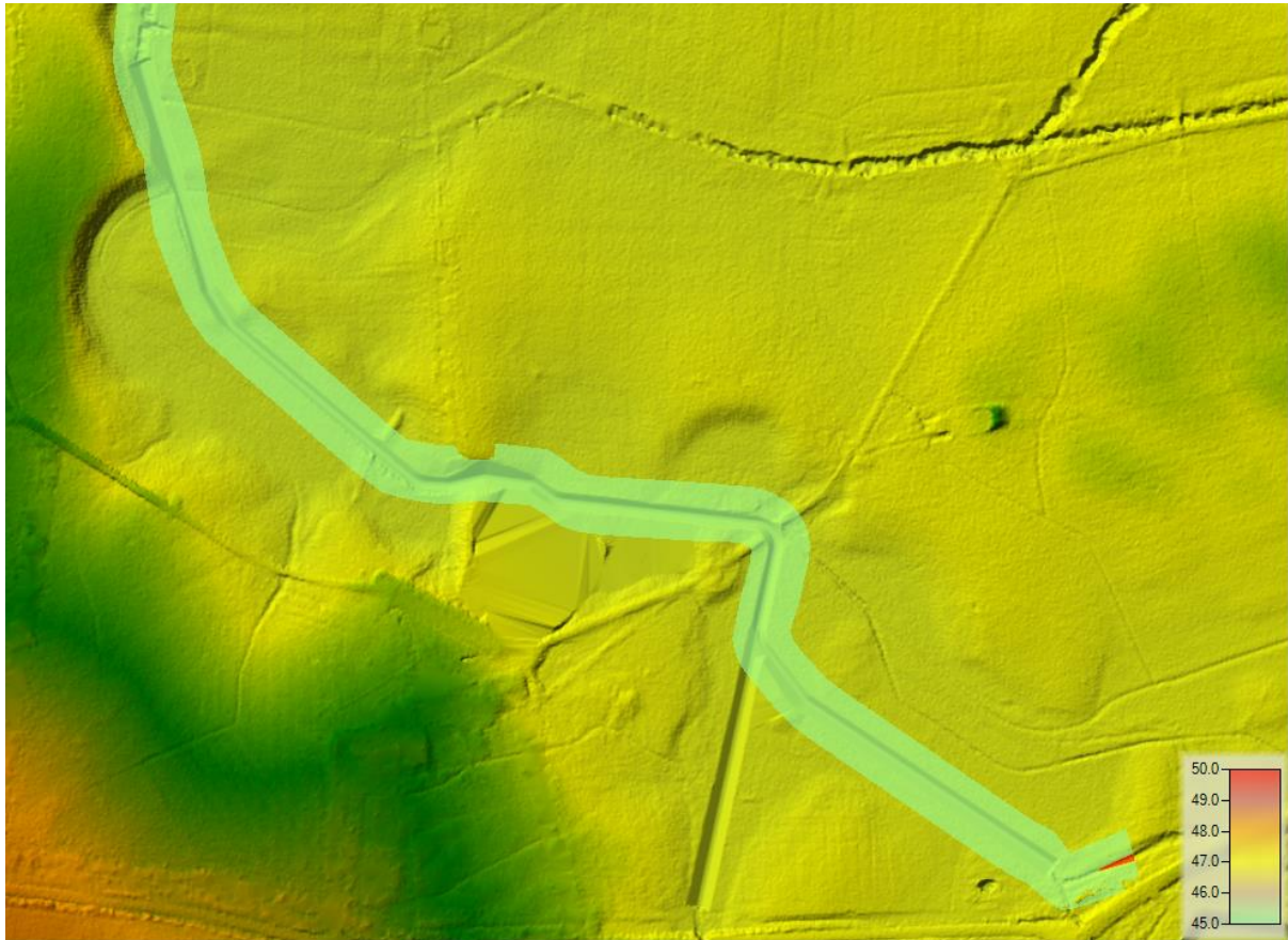
Figure 55. Average shear stress map through constructed waterway (in N/m^2 ) – note red grading near WLRB1 (DCP ref WL-01) outfall to MOP.
