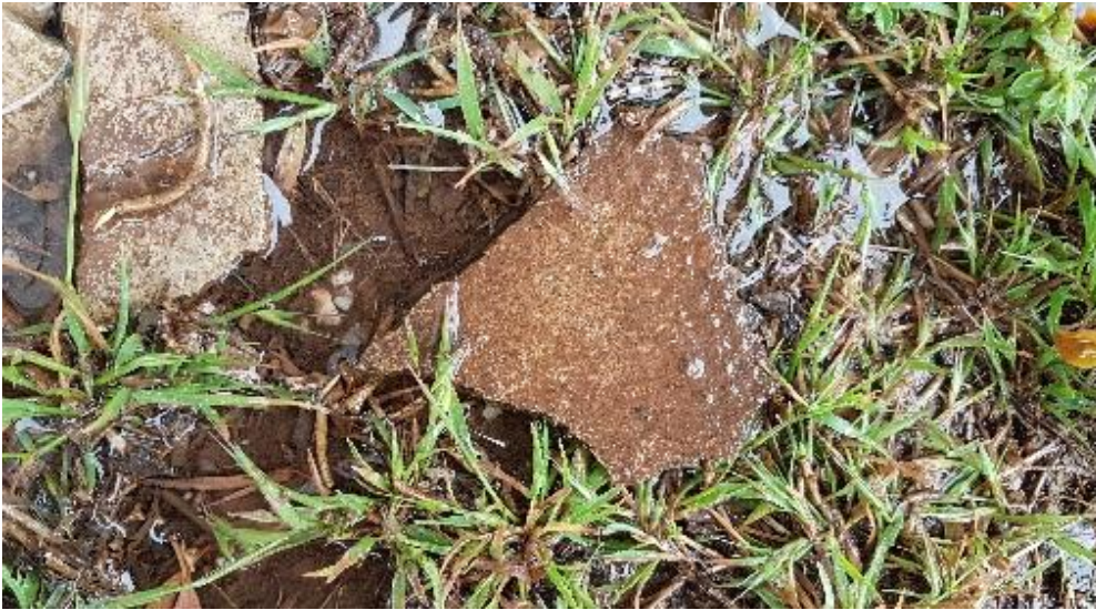
Figure C.5 : Suspected ACM observed at AOI 3 (16/11/17)
