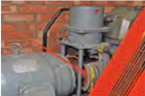
Asbestos brake lining on output shaft of AC motor (friable)
