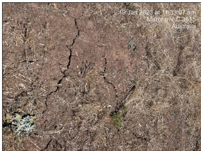
Photo 7.3 Minor surface cracking observed within Quaternary Colluvium.
