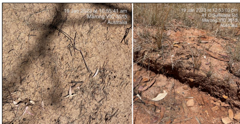
Photo 7.2 Examples of observed surface geology. Left: clayey silt. Right: silty sand with clay and gravel.
