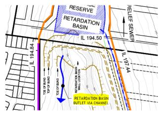
Preliminary advice from MWC indicates a sediment pond will be located on AHCEV land directly to the north west of NH04 to treat water flowing into the retarding basin and creek. The Stormwater Quality assets proposed within the Yuroke Creek DSS area are subject to change based on the detailed design and consultation with Melbourne Water's Drinking Water Quality team.
