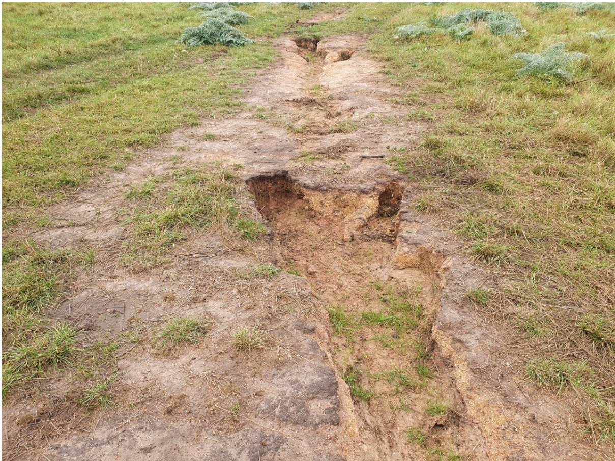
Photograph 13: View of the soil profile within the onsite track in the southern portion of the site. Sandy clay fill material was present within the track.
