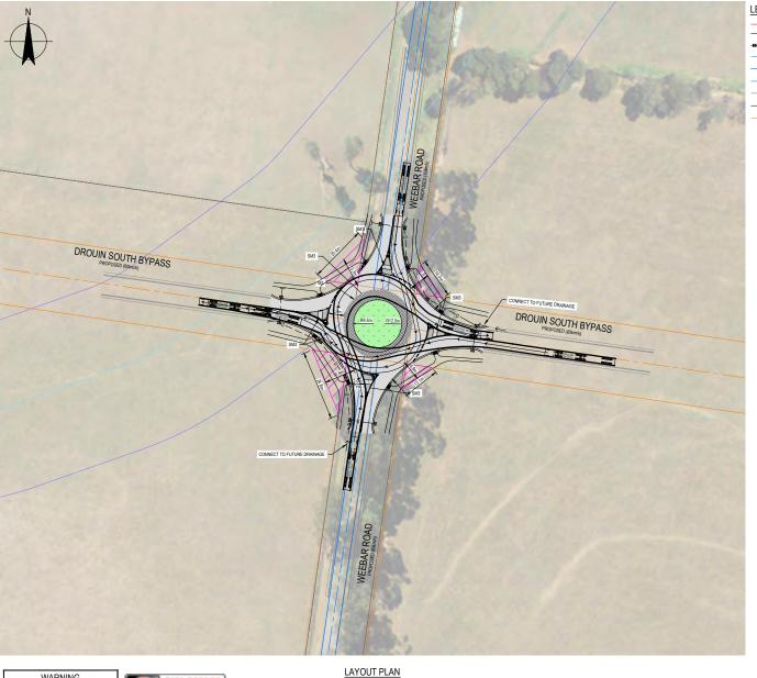
LEGEND PROPOSED LAND ACQUISITION PROPOSED ROAD CENTRE LINE PROPOSED INVERT OF KERB ■ D — PROPOSED DRAINAGE PROPOSED MOUNTABLE CONCRETE APRON EXISTING ROAD CENTRE LINE PROPOSED GRASSED AREA PROPOSED ROAD PAVEMENT EXISTING WATER WAY PROPOSED ROAD RESERVE
