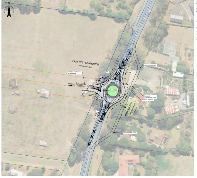
LEGEND PROPOSED ROAD CENTRE LINE OPEN PASSIVE RESERVE PROPOSED INVERT OF KERB NATIVE VEGETATION RESERVE PROPOSED DRAINAGE RECREATION RESERVE ---- PROPOSED SWALE EXISTING ROAD CENTRE LINE PROPOSED LAND ACQUISITION EXISTING LINE MARKING EXISTING TRAIN TRACK PROPOSED MOUNTABLE CONCRETE APRON APPROVED PARCEL PROPOSED GRASSED AREA PROPOSED ROAD PAVEMENT EXISTING WATER WAY PROPOSED ROAD RESERVE
