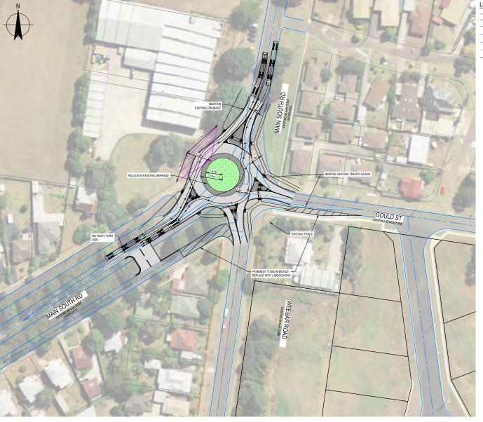
**LEGEND** PROPOSED ROAD CENTRE LINE PROPOSED TRAFFIC ISLAND PROPOSED INVERT OF KERB PROPOSED MOUNTABLE CONCRETE APRON EXISTING ROAD CENTRE LINE EXISTING KERB PROPOSED GRASSED AREA EXISTING LINE MARKING PROPOSED ROAD PAVEMENT PROPOSED PARCEL
