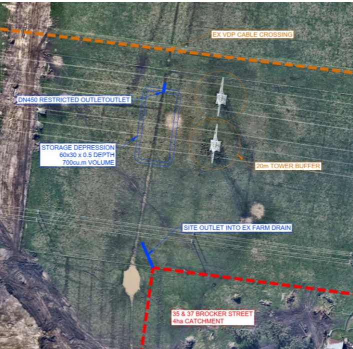
Figure 9: Alternative Drainage Outfall
