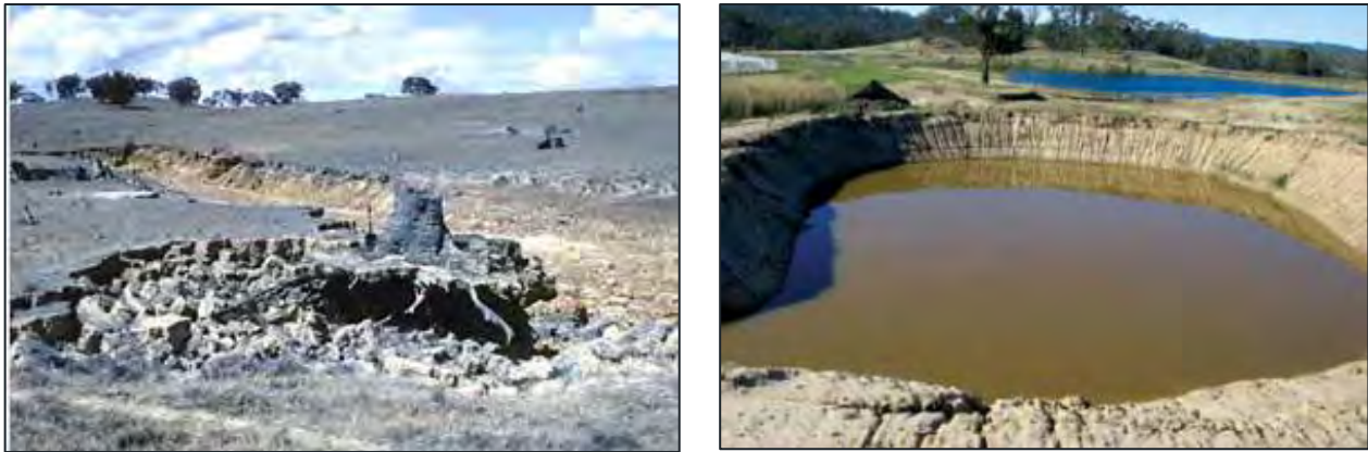
Figure 2.2 Tunnel erosion of dispersive clay subsoil, https://vro.agriculture.vic.gov.au (accessed 2024) (Left), and construction of dam in dispersive soils leading to rill erosion, https://nre.tas.gov.au (accessed 2024) (Right)
