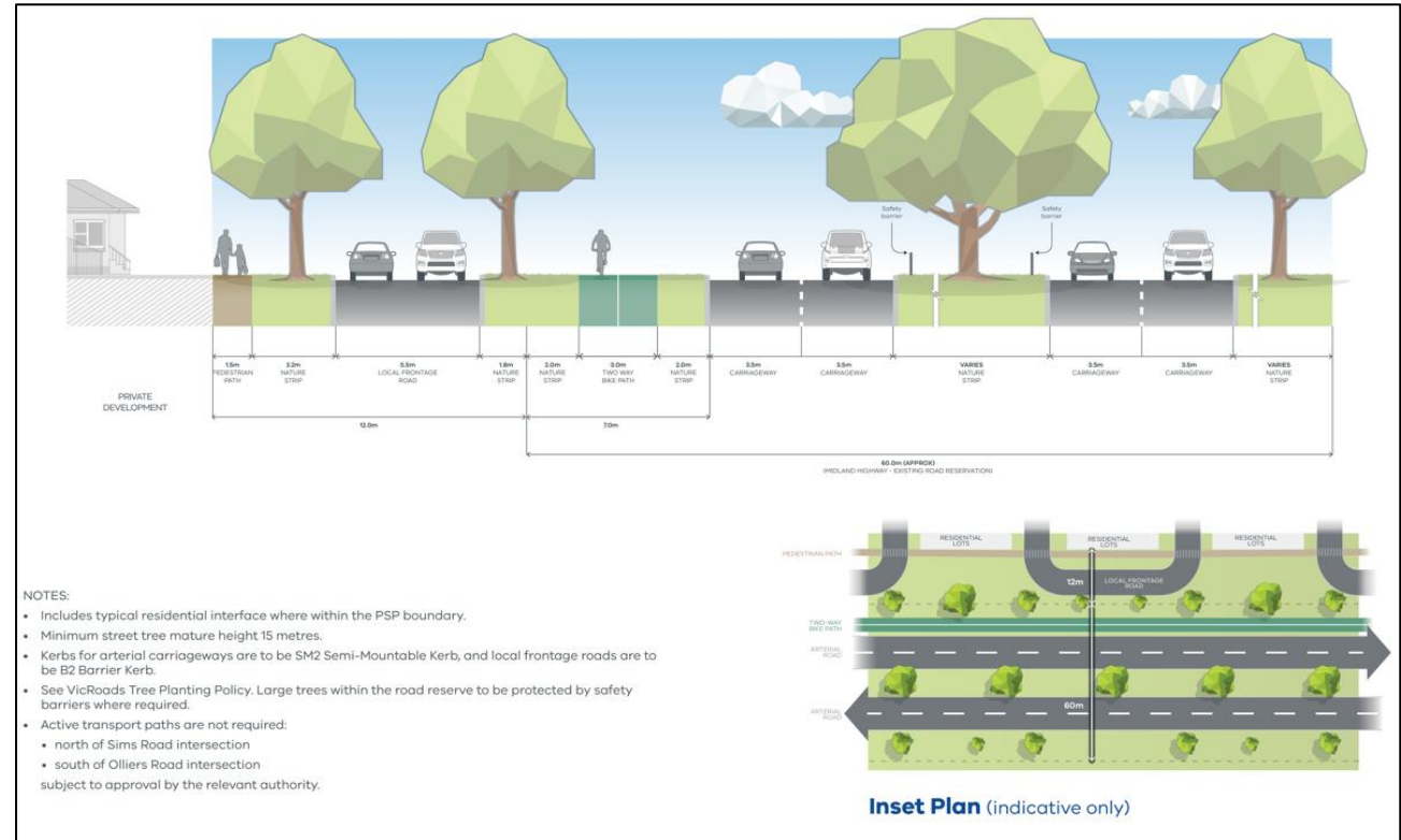
Figure 6-7. Primary arterial cross section, Midland Highway – 60m (Source: VPA)
