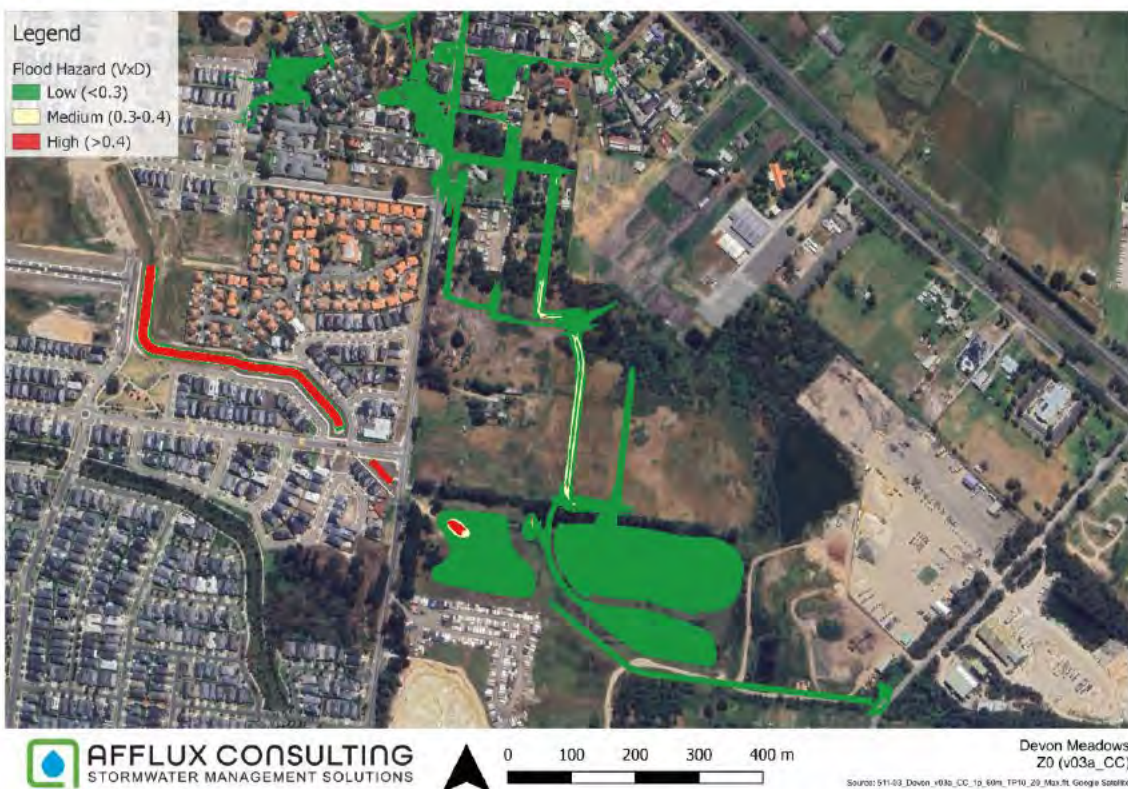
Figure 12. DELWP Flood hazard rating for post-development with v4.1 climate change scenario (18.5% flow increase)
