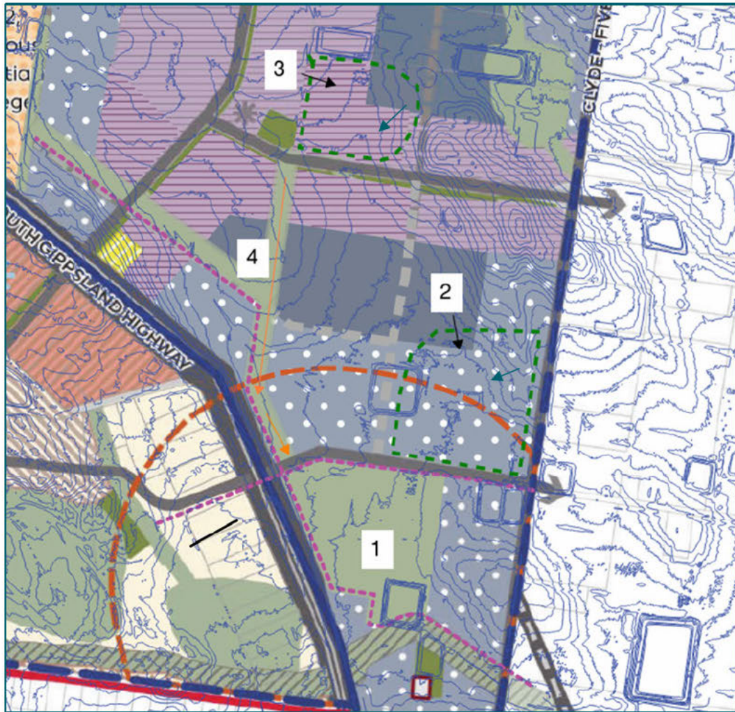
Figure 4: Alternative Drainage Concept with contours - indicating levels within the Draft PSP wetlands shown by green dash
