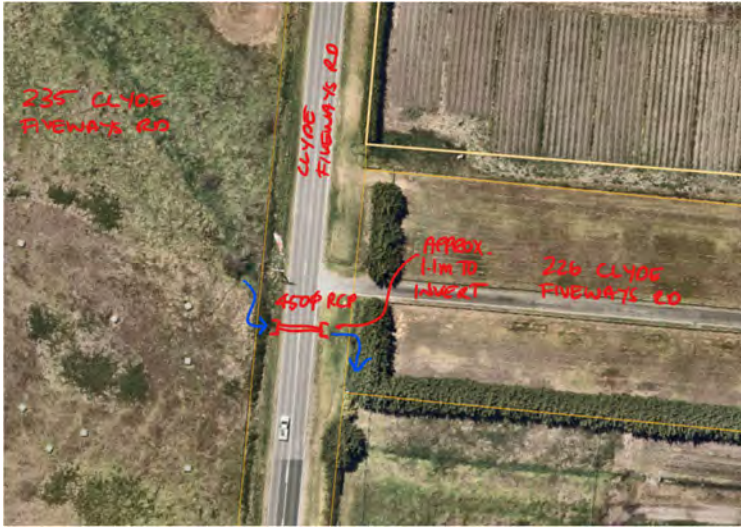
Figure 5 - Existing outfall arrangements downstream of CFS3
