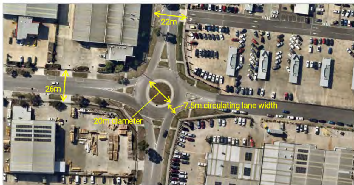
Figure 11: Industrial Estate Cross-Intersection Roundabout Example – Pakenham
