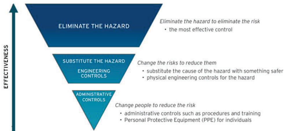
Figure 3-1 Hierarchy of controlling hazards
