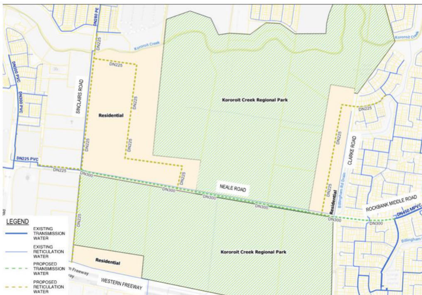
Figure 3 Potable water future servicing plan (GWW, 2025)
