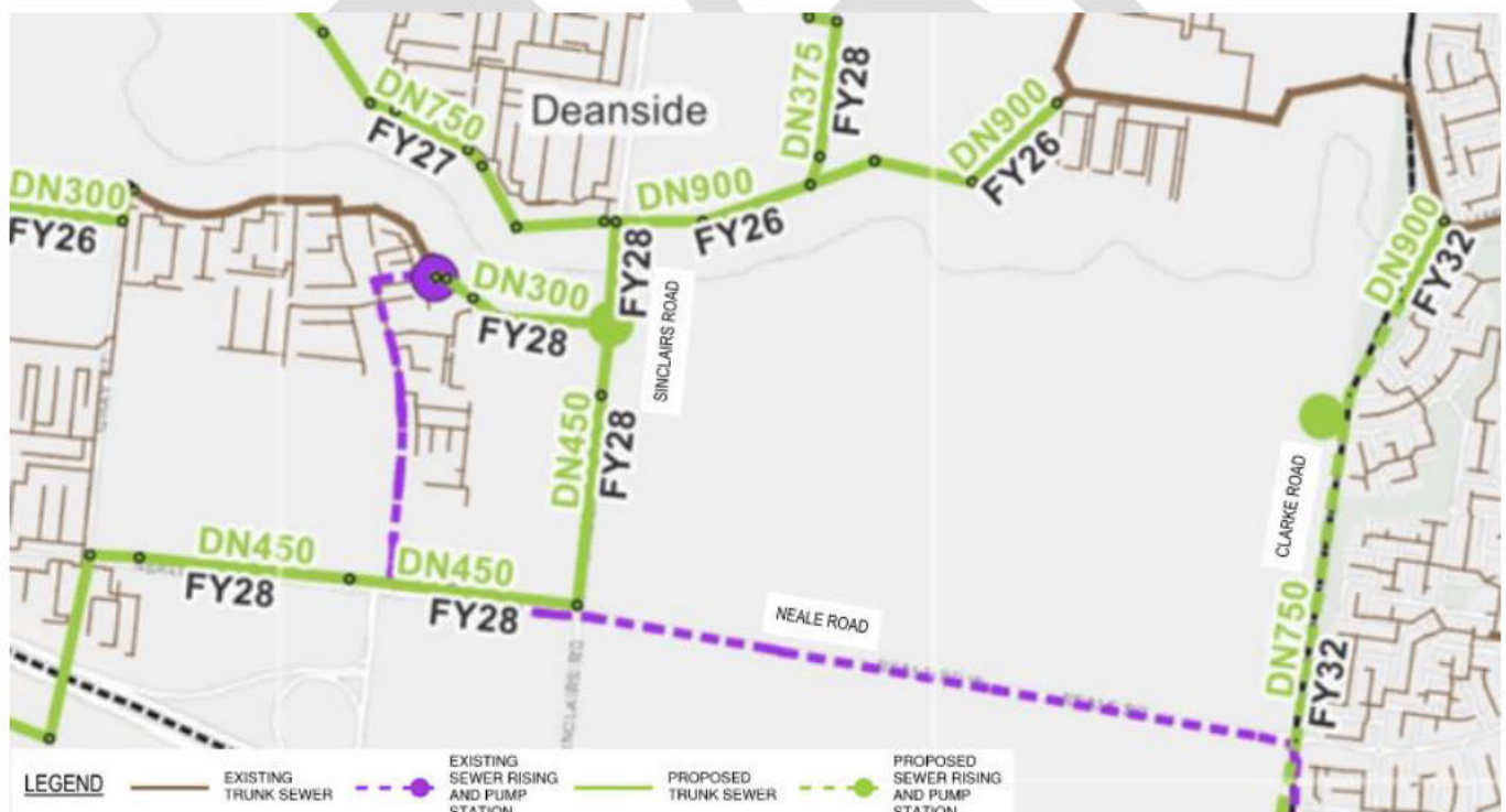
Figure 4 Sewer future servicing plan (GWW, 2025)
