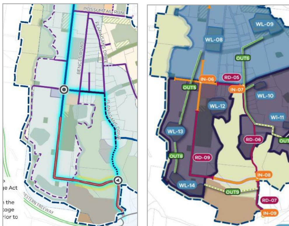
Figure 2 - Drainage outfalls OUT5 and OUT6 not aligned with the local road network
